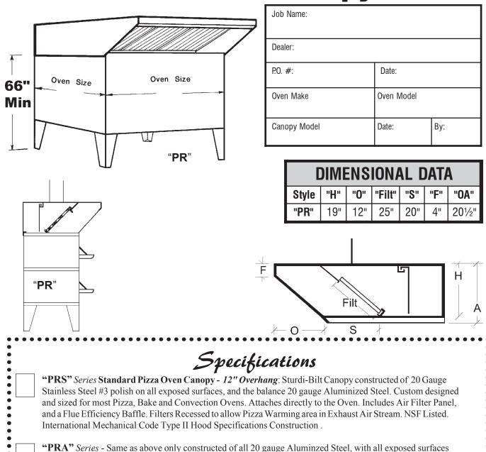
"PR96" Series - NFPA #96 18 Ga Construction, all externally welded construction, Aluminum Baffle Grease Filters, International Mechancial Code Type I Hood Construction, available S/S or Painted Aluminzed Steel
