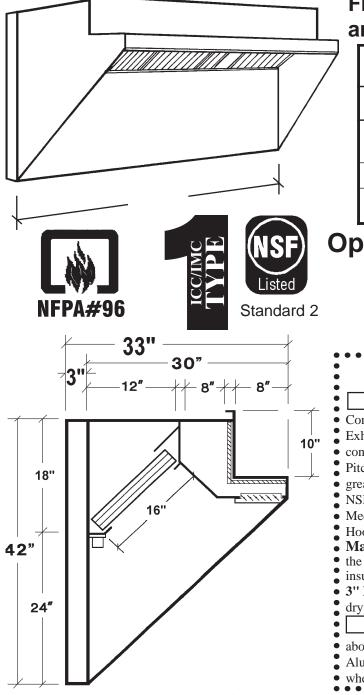
Front Untempered Make Up Air and 3" NFPA #96 Air Space
